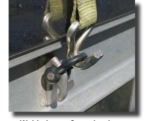
Welded rope & eye hooks
